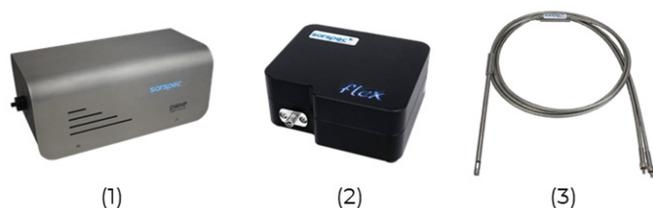
**Figure 2** – W20 Light source (1), FLEX spectrometer (2), and transmission probe (3) were used to evaluate the transmittance spectra and CIELAB color coordinates of red cabbage extract.
