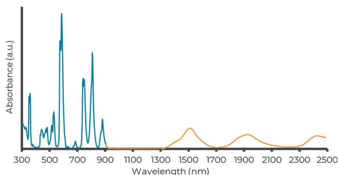
**Figure 4** – Absorption spectrum of didymium glass filter obtained with FAbS from 300 to 900 nm (blue line), and ProNIR from 900 to 2300 nm (yellow line).
