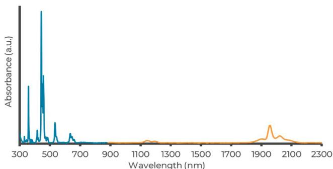
**Figure 3** – Absorption spectrum of holmium glass filter obtained with FAbS from 300 to 900 nm (blue line), and ProNIR from 900 to 2300 nm (yellow line).
