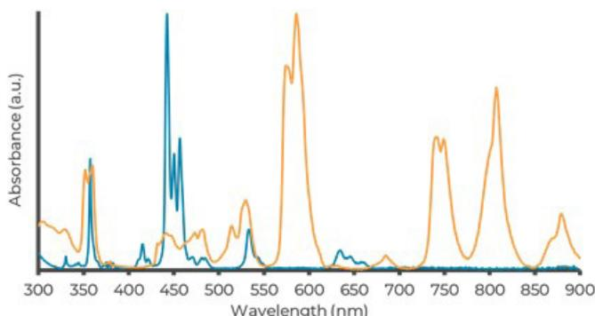
**Figure 2** – Normalized absorption spectra of holmium (blue line) and didymium (yellow line) glass filters, previously obtained with the new FAbS spectrophotometer.
