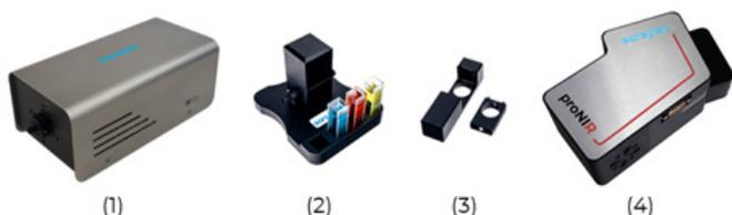
**Figure 1** – W20 Light source (1), Standard Cuvette Holder (2), Solid Sample Holder (3), ProNIR Spectrometer (4) used to measure the NIR absorption spectra of holmium and didymium glass filters.
