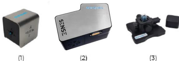
**Figure 2** – LED Light source (1), SENSE spectrometer (2), and multipurpose cuvette holder (3) were used to determine the concentration of quinine in tonic water samples.
