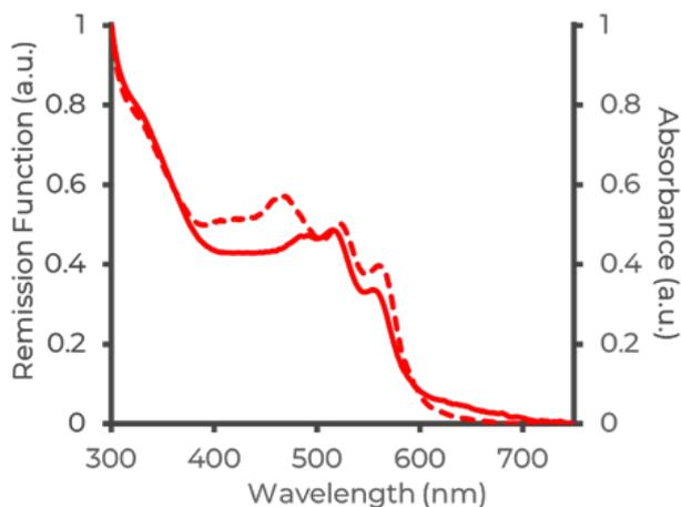
**Figure 7** – Remission function  $F(R_{\infty})$  as derived by equation 1 for (a) blue, (b) green and (c) red dyes obtained by ground-state diffuse reflectance technique (dash line), given in Figure 6. The absorption spectra of the corresponding dye solutions (solid line) were added for a peak structure and wavelength comparison.
