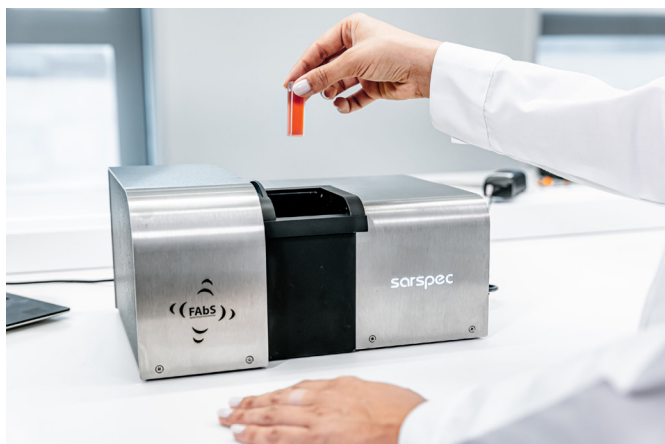
Figure 4 – The FAbS spectrophotometer was used to measure the absorption spectra of both reference and sample xanthene dyes.
