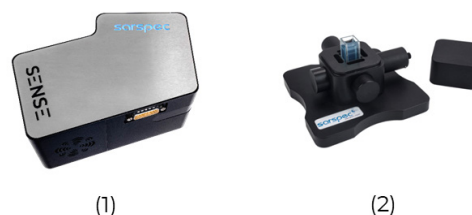
Figure 3 – SENSE spectrometer (1), and multipurpose cuvette holder (2) were used to measure the fluorescence quantum yield of some xanthene dyes.
