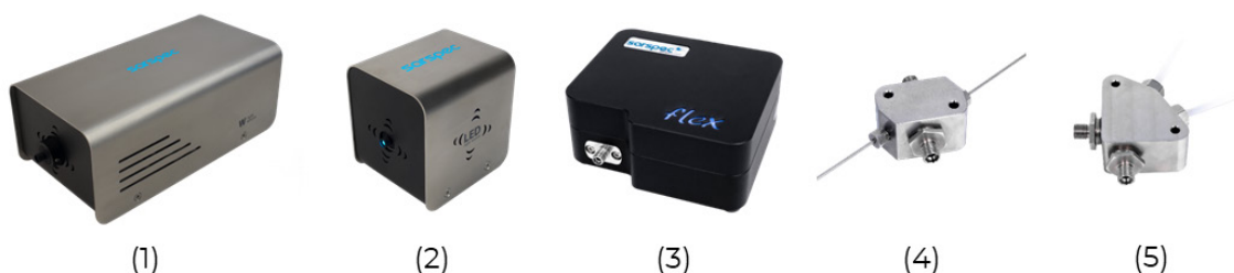
Figure 2 – W20 light source (1), LED light source (2), FLEX RES spectrometer (3), and absorbance (4) and fluorescence (5) flow cells were used to assess the pH-dependence of the absorption and fluorescence spectra of fluorescein.
