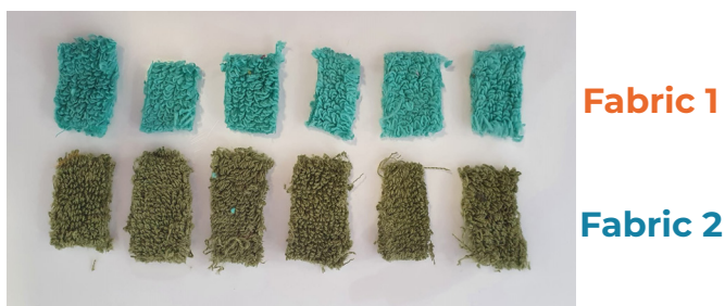
Figure 4 – The reflectance spectra and L*a*b* color coordinates were measured for six samples of the two fabrics.
